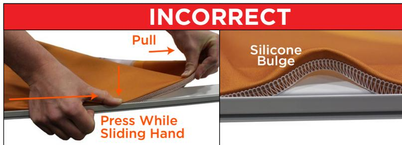
Pulling on the silicone welt during installation stretches the silicone and creates a bulge in the silicone welt that is difficult to correct smoothly.
