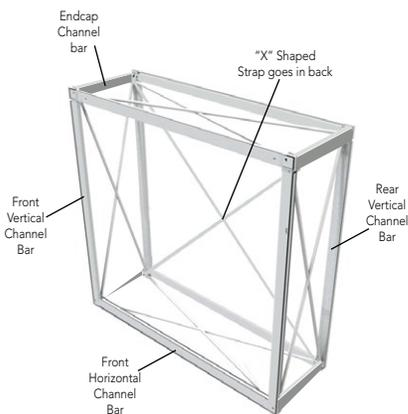
Diagram showing the locations of the channel bars required.
