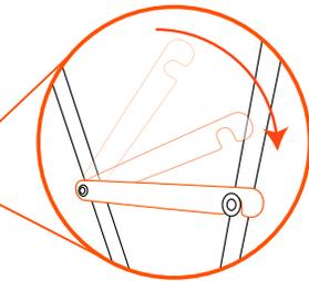
2. Lock the two metal support brackets to secure the frame open.
