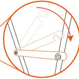
2. Lock the two metal support brackets to secure the frame open.
