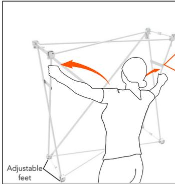
1. Expand the frame with the adjustable feet pointed down.
