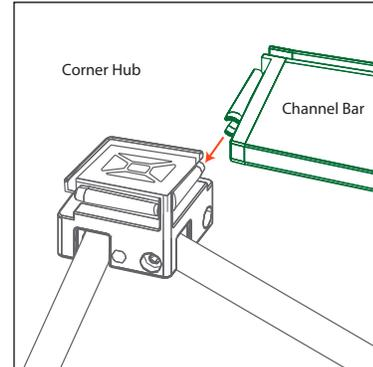
3. Install the 4 front channel bars and rear 4 back channel bars. The thinner edge goes toward the inside of the frame.
