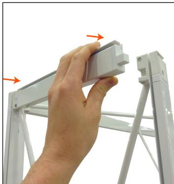
4. Snap the four endcap channel bars to the top and bottom sides of the frame.
