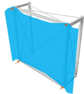
5. Install the wrap-around fabric graphics. See the following page for detailed graphic installation.
