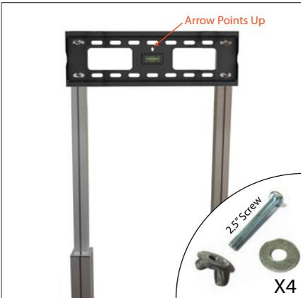
4. Install monitor mount plate with 2.5" screws, small washers, and wing nuts. Level bracket by adjusting the column heights. Tighten adjustment knobs and bracket screws.
