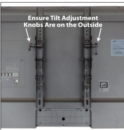
6. Install monitor brackets to the back of the monitor using appropriate screws, washers, and optional spacers for the monitor you are using. See instruction manual included with the monitor bracket for details. *Note: We recommend monitors that do not exceed 50 lbs.*
