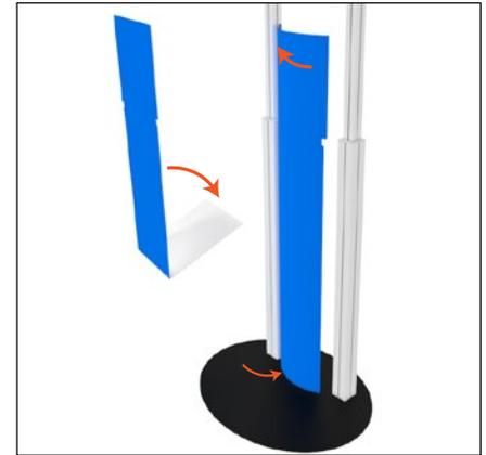
3. Unfold optional graphic infill. Place one graphic edge in column channel. Slightly bend graphic and tuck opposite side in opposite column channel.
