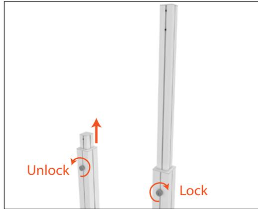
2. Loosen height adjustment knobs and extend columns to desired height. (60" from the ground is recommended)
