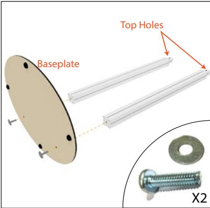
1. Connect column pieces to baseplate with two large screws and large washers. Make sure the adjustable knobs are pointed towards the rear. Stand the display up.
