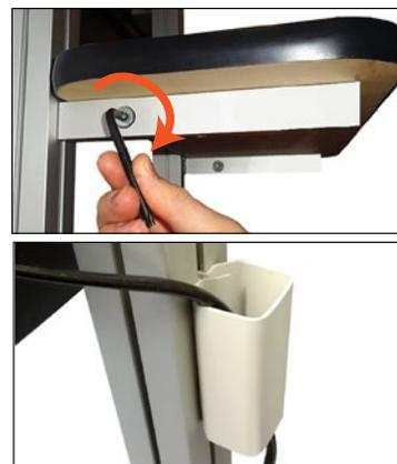
8. Attach the shelf in the desired location using the star bit wrench. Cable clips may be used for holding wires out of the way.
