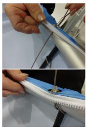
8. Feed the other end of the wire through the grommet in the outside of the graphic. Continue zipping the graphic up. Each time you reach a grommet, feed the wire through.
