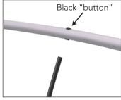
5. The other end of vertical shaft goes into top rectangle. Press down firmly on frame to ensure poles are fully seated.
