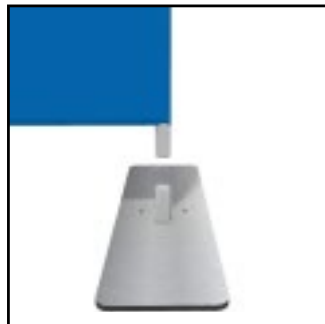
6b. If your kit includes a single foot, attach it to bottom of frame. Secure foot with locking pin.
