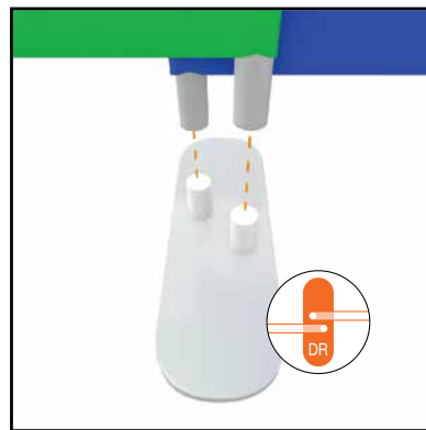
7c. If your kit includes a double foot labeled (DR), connect as seen above. Frame on left (shown in green above) attaches to the front foot nub and overlaps the back frame by approximately 3.5 inches.
