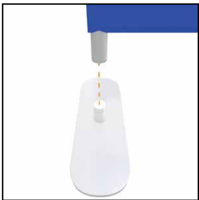
7a. Attach feet to bottom of frames. Secure foot with locking pin.
