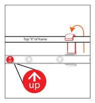
7. With the "up" sticker facing toward the top of the frame, mount the clips to the frame so the hooks are facing the front. Stretch the bottom hooks down and hook them onto the bottom of the frame.
