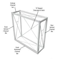
Diagram showing the locations of the channel bars required.
