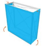
3. Wrap the endcap around the sides of the counter and tuck into the rear side vertical SEG grooves.
