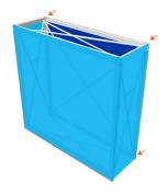
4. Install the back graphics by first tucking all four corners into the rear-facing SEG grooves. Then, tuck the remaining silicone into the SEG grooves.
