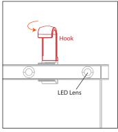
6. Rotate the hooks to face the same direction as the LED lenses.
