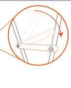
2. Lock the two metal support brackets to secure the frame open.
