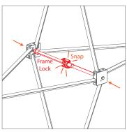
2. Snap all frame locks (marked in red in the diagram above) to secure the frame.
