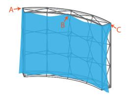
A. Tuck the graphic into left/upper endcap SEG channel D. Complete installation of the top and partially down the vertical channel bar. B. Holding the graphic off of the ground, tuck the center of the graphic on the front of the frame. C. Tuck the graphic into the right endcap.
