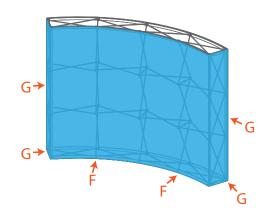
F. Complete installation on the bottom/front. G. Complete installation of both endcaps.
