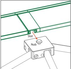
channel bar onto the nubs on the hubs.
