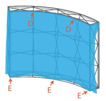
edge of the graphic. E. Tuck the bottom/front corners and the middle of the bottom/front.
