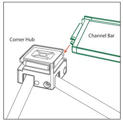
4A. Slide one end of the first channel bar 4B. Snap the slots in the back of the onto the connection point of one of the corner hubs.
