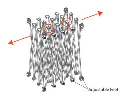
1. Set the frame standing on end. Grasp two of the middle hubs (circled in orange) and gently expand the frame. Note the location of the adjustable feet for future reference.
