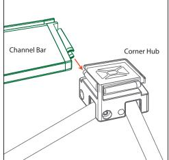
4C. Attach the other end of the channel bar to the other corner hub. Repeat steps 4A-4C for all channel bars as seen in the diagrams above.
