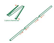
3. Unfold and slip together each bungeed channel bar.
