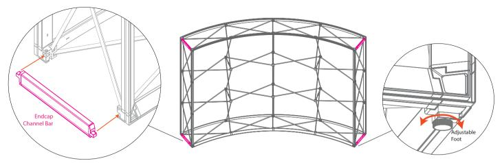
5. Snap four endcap channel bars onto the sides of the frame.
