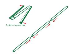
3. Unfold and slip together each bungeed channel bar.
