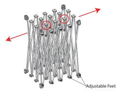
1. Set the frame standing on end. Grasp two of the middle hubs (circled in orange) and gently expand the frame. Note the location of the adjustable feet for future reference.
