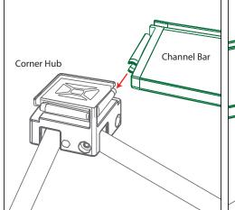
4A. Slide one end of the first channel bar onto the connection point of one of the corner hubs.
