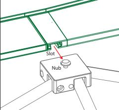
4B. Snap the slots in the back of the channel bar onto the nubs on the hubs.
