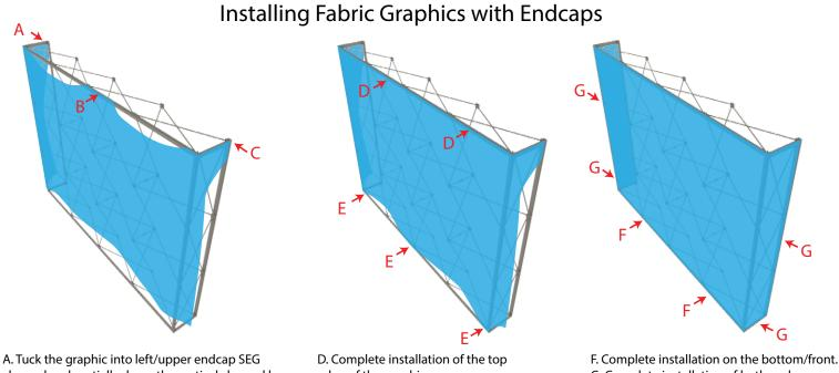
channel and partially down the vertical channel bar. B. Holding the graphic off of the ground, tuck the center of the graphic on the front of the frame. C. Tuck the graphic into the right endcap.
