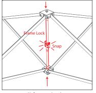
2. Snap all frame locks (marked in red in the diagrams below) to secure the frame.
