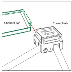
4C. Attach the other end of the channel bar to the other corner hub. Repeat steps 4A-4C for all channel bars as seen in the diagrams above.
