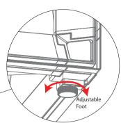
7. If the frame is on an uneven floor or if it leans, adjust the bottom feet.
