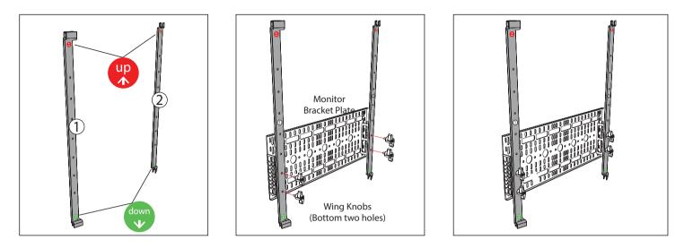
1. Attach the monitor bracket plate to the two vertical pieces with four wing knobs. The wing knobs will go through the bottom two mounting holes in the vertical pieces Note the up and down arrows on the vertical pieces.
