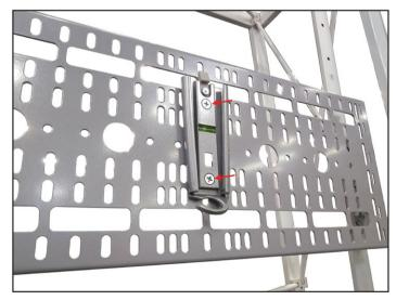
5. Attach the smaller monitor bracket back plate onto the monitor bracket plate as seen above using the provided screws and wing-nuts.
