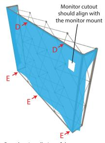
D. Complete installation of the top edge of the graphic. E. Tuck the bottom/front corners and the middle of the bottom/front.
