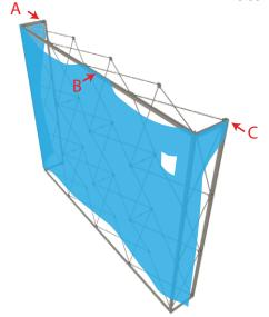
A. Tuck the graphic into left/upper endcap SEG channel and partially down the vertical channel bar. B. Holding the graphic off of the ground, tuck the center of the graphic on the front of the frame. C. Tuck the graphic into the right endcap.
