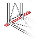
2. Slide the stabilizing foot back and slide the same socket over the back adjustable foot.
