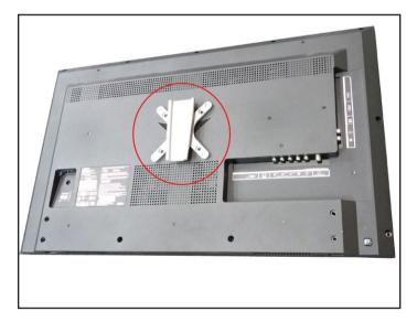
6. Attach the X-shaped monitor mount to the television using the appropriate screws for the television. The bracket is compatible with VESA 75 (inner mounting holes) and VESA 100 (outer mounting holes).
