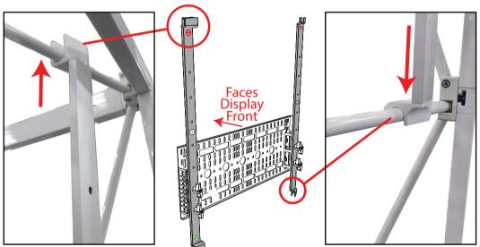
2. To hang the monitor bracket plate onto the frame, slide the upper u-channels over the top cross member of the frame.
