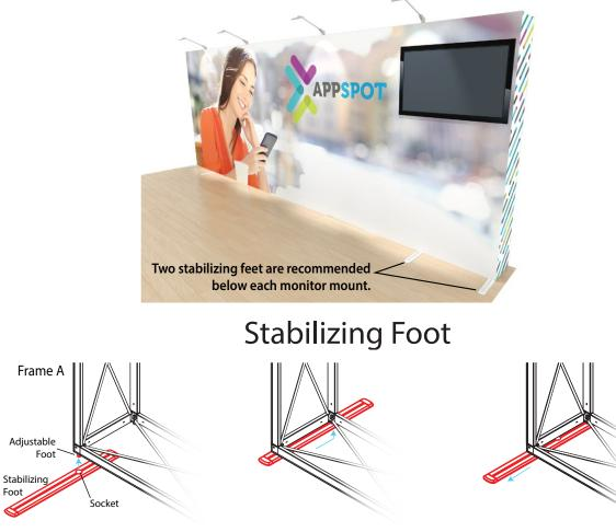
1. Slide the socket of the stabilizing foot over the front adustable foot of the frame.
