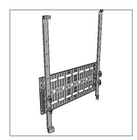
4. Attach the monitor bracket plate to the two vertical pieces with four wing knobs. The wing knobs will go through the bottom two mounting holes in the vertical pieces Note the up and down arrows on the vertical pieces.
