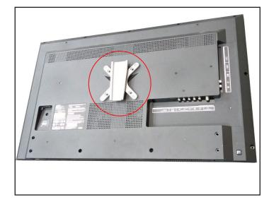
4. Attach the X-shaped monitor mount to the television using the appropriate screws for the television. The bracket is compatible with VESA 75 (inner mounting holes) and VESA 100 (outer mounting holes).
