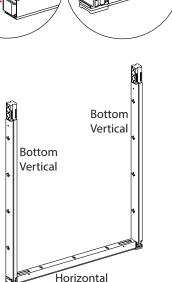
vertical bars, lift the lock lever, slide the parts together, and close the lock lever.
