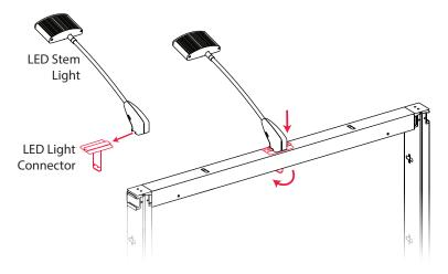
Attach the LED Stem Light to the LED Light connector (marked in red).
