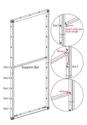
3. Attach the support bar by inserting the non-spring-loaded end into the 5th slot on the left with the other end of the bar lifted. Retract the spring lock and lower the right side until it lines up with the right slot. Release the spring lock.
