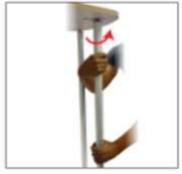
4. Place the counter base on top of the support poles. While holding the bottom pole, hand-tighten the top pole into the base.
