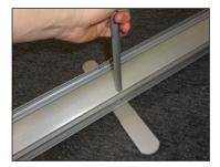
Extend bungied pole and insert into hole in base.
