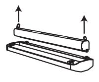
2. Pull up on the tabs to remove the graphic cartridge
