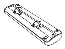
1. Flip the base over and rotate the two locks counter-clockwise.
