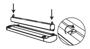
3. Insert the new graphic cartridge and rotate the locks clockwise to secrue.
