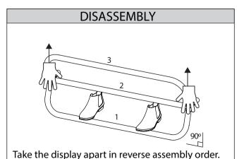
If it is difficult to disassemble the base, place feet as shown above. Pull up at both ends of pole 2 to remove pole 1. Pull with even pressure. Flip the part and repeat to remove tube 3.
