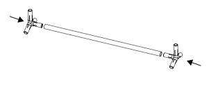
1. Begin building the center of the base by installing the corner pieces on each end of the center base pole.
