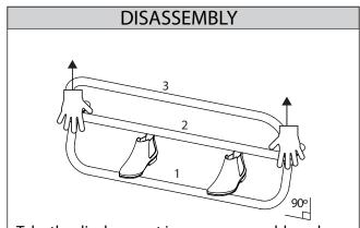
Take the display apart in reverse assembly order. If it is difficult to disassemble the base, place feet as shown above. Pull up at both ends of pole 2 to remove pole 1. Pull with even pressure. Flip the part and repeat to remove tube 3.
