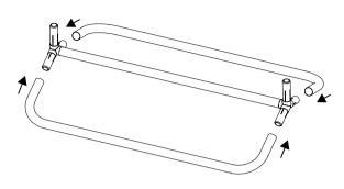
2. Complete the base assembly by adding the two poles with curved ends.
